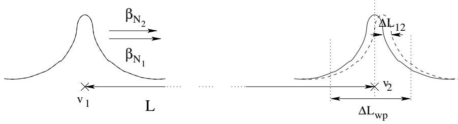
FIGURE 5.3: Graphical representation of the hierarchy Eq. (5.30) of the lengths \Delta L_{12} , \Delta L_{\text{wp}} and the detector length L . The two interaction vertices (the production and the decay vertex of the neutrino N ) are denoted as v_1 and v_2 , respectively. Note that at the production vertex ( v_1 ) the wavepackets of N_1 and N_2 are not mutually displaced, unlike in the decay vertex ( v_2 ).
